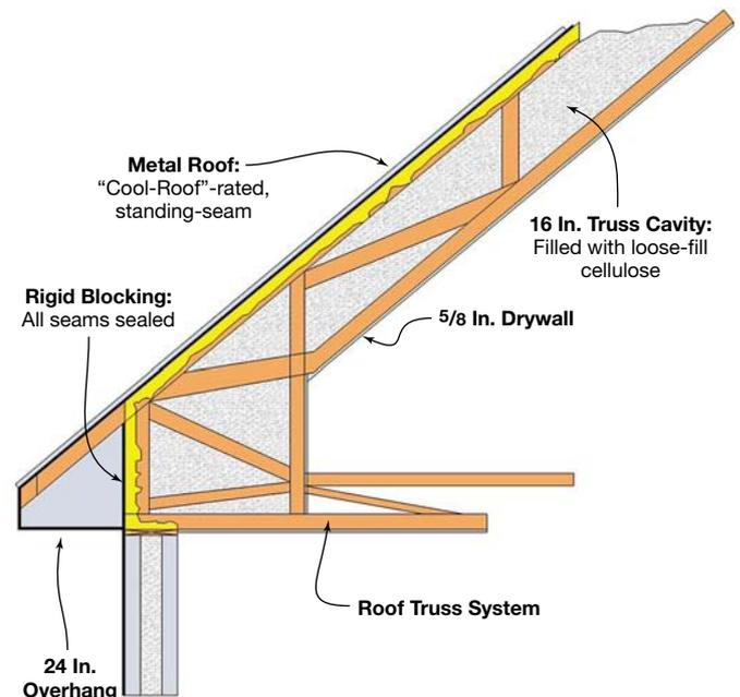
**Air Sealing & Ventilation.** The house’s airtight design is aided by the barrier layer of spray foam inside the entire shell. The use of a condensing, non-vented clothes dryer and a recirculating range hood also helps keep the thermal boundary tight and eliminate pressure imbalances.
