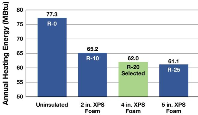
**Slab insulation** analysis came first and the resulting graph shows the change in annual heating energy for incrementally higher levels of perimeter and under-slab insulation. The slab thickness is fixed at four inches to balance thermal mass and thermal lag. As shown, the impact of slab insulation is greater from R-0 to R-10 and begins to level off at R-20. As a balance between cost and performance, we chose R-20 for both the perimeter and under the slab.
