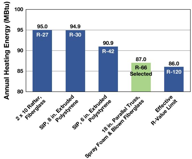
**Roof analysis** was similar to the walls with its hypothetical R-120 value for an upper limit. We could not meet our R-60 roof goal with SIPs. The highest-performing panel, a 12-inch-thick extruded polystyrene, reached R-57 and was significantly more expensive than other alternatives. We transitioned to a new plan—a parallel truss system.
