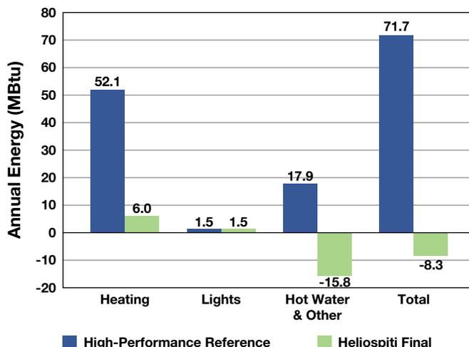
comparison just reflects the effects of insulation, air sealing and passive solar design (passive thermal losses and passive solar gain) with the reference house.
