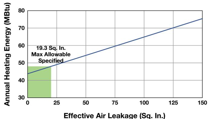
square inches of effective leakage area. Although our target is an aggressive air leakage limit, the passive house community has shown that even more stringent limits can be reached. Of course, this level of air-tightness necessitates mechanical whole-house ventilation.
